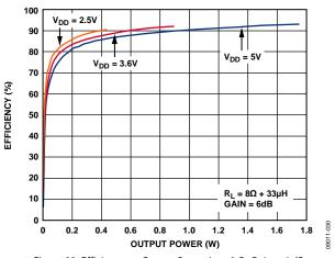
Figure 23. Efficiency vs. Output Power into 8  $\Omega$ , Gain = 6 dB
