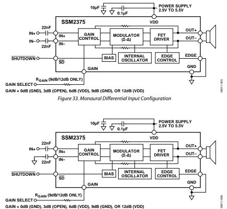
GAIN = 0dB (GND), 3dB (OPEN), 6dB (VDD), 9dB (GND), OR 12dB (VDD)
