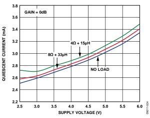
Figure 17. Quiescent Current vs. Supply Voltage, Gain = 0 dB
