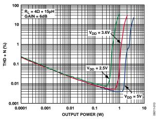
Figure 4. THD + N vs. Output Power into 4  $\Omega$ , Gain = 6 dB
