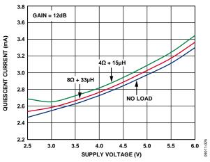
Figure 20. Quiescent Current vs. Supply Voltage, Gain = 12 dB
