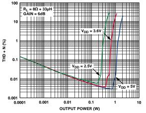
Figure 3. THD + N vs. Output Power into 8  $\Omega$ , Gain = 6 dB
