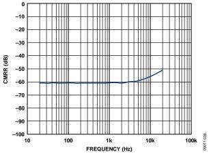
Figure 28. Common-Mode Rejection Ratio (CMRR) vs. Frequency
