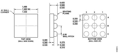
Figure 36. 9-Ball Wafer Level Chip Scale Package [WLCSP] (CB-9-2) Dimensions shown in millimeters
